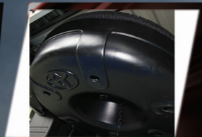
SPARE WHEEL COVER This product conceals the spare wheel under the vehicle and protects it from unnecessary travel wear.
